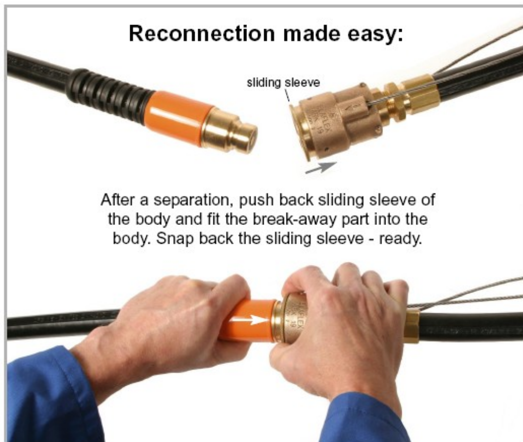
Fig. 14 - ARK 19 reconnectable hose break-away valve
