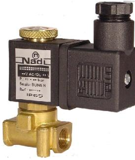
Two way direct acting solenoid valve with spring return.
