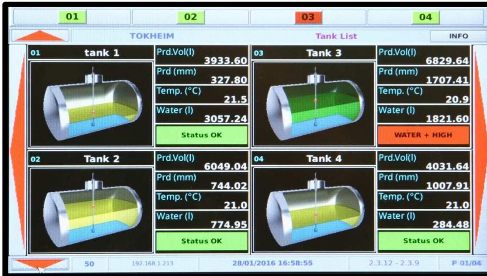
This page summarizes the main information relating to one or more tanks. You can view up to 4 tanks simultaneously on the same page. If there are more than 4 tanks configured you can view the next one by pressing the large red arrows in the left and right parts of the page.
