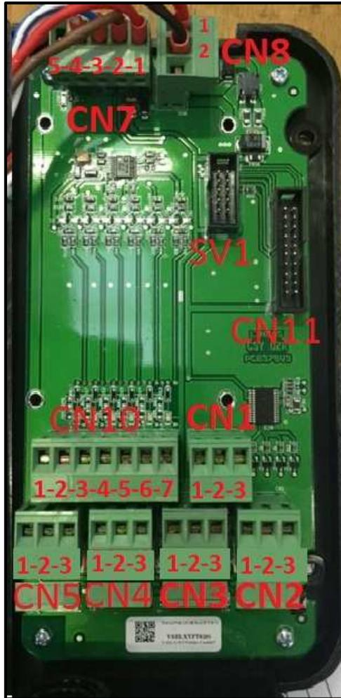
The XMT model explosion probes must be connected in parallel to the console and directly to the connector CN7 *without* passing through the intrinsically safe barrier. In this case the barrier remains unused.
