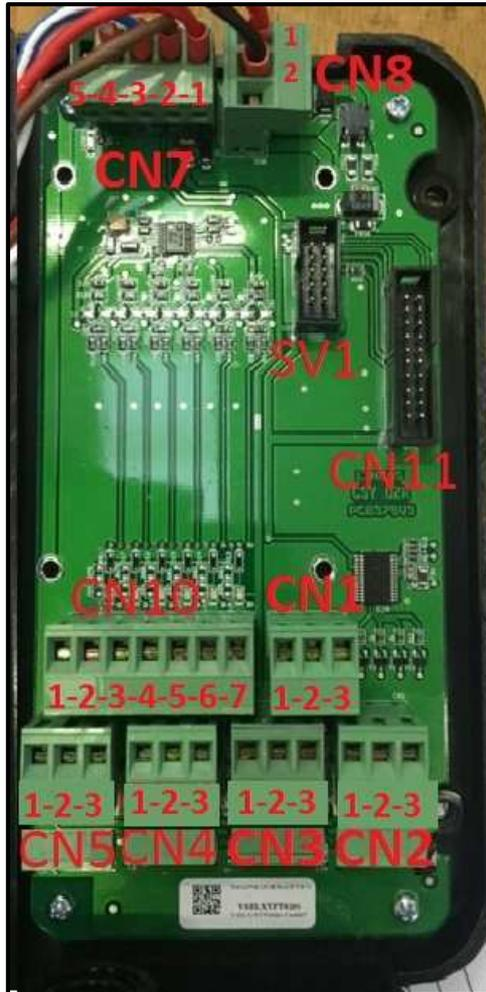
The receiver connects directly to connector CN7 without going through the intrinsically safe barrier. In this case the barrier remains unused.
