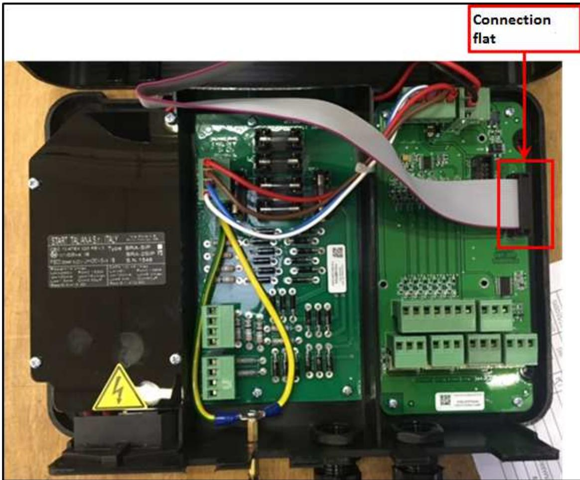
After disconnecting the ribbon cable fix the rear part to the wall (We recommend using Fischer dowels, size 6). The following image shows the mounting holes:
